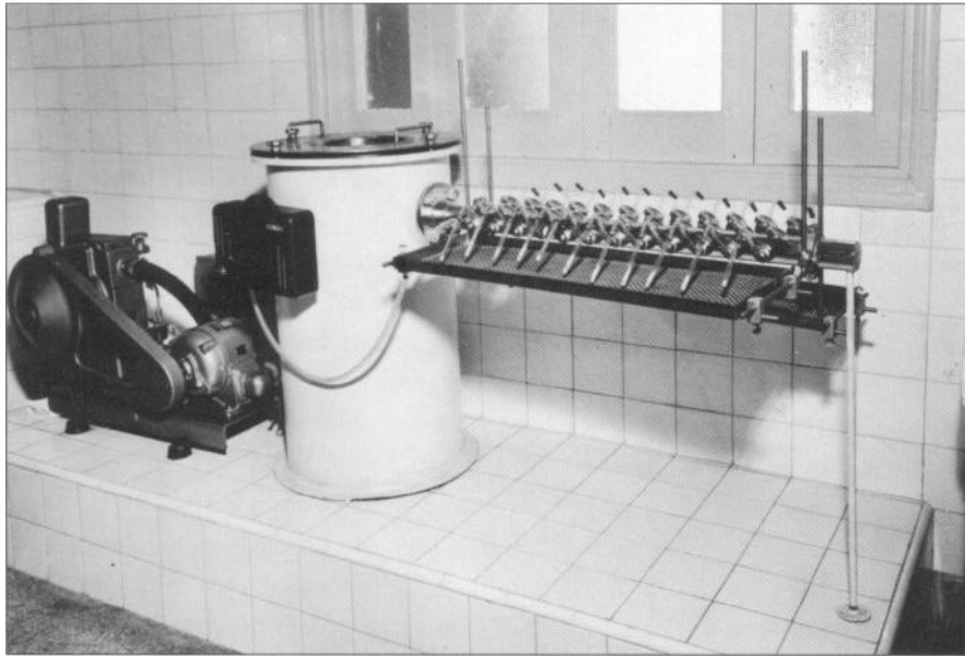
A freeze-drying unit for the production of smallpox vaccine, Institute of Hygiene, Havana, Cuba, 1956. Freeze-dried vaccine remained effective without refrigeration even in tropical heat, and its production in several countries of the Americas, facilitated by PAHO-supplied equipment and consultants, aided the smallpox eradication campaign in this Hemisphere.
