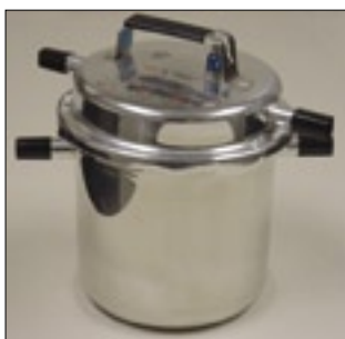
FIGURE 17. Autoclave: high-pressure, saturated steam sterilization
