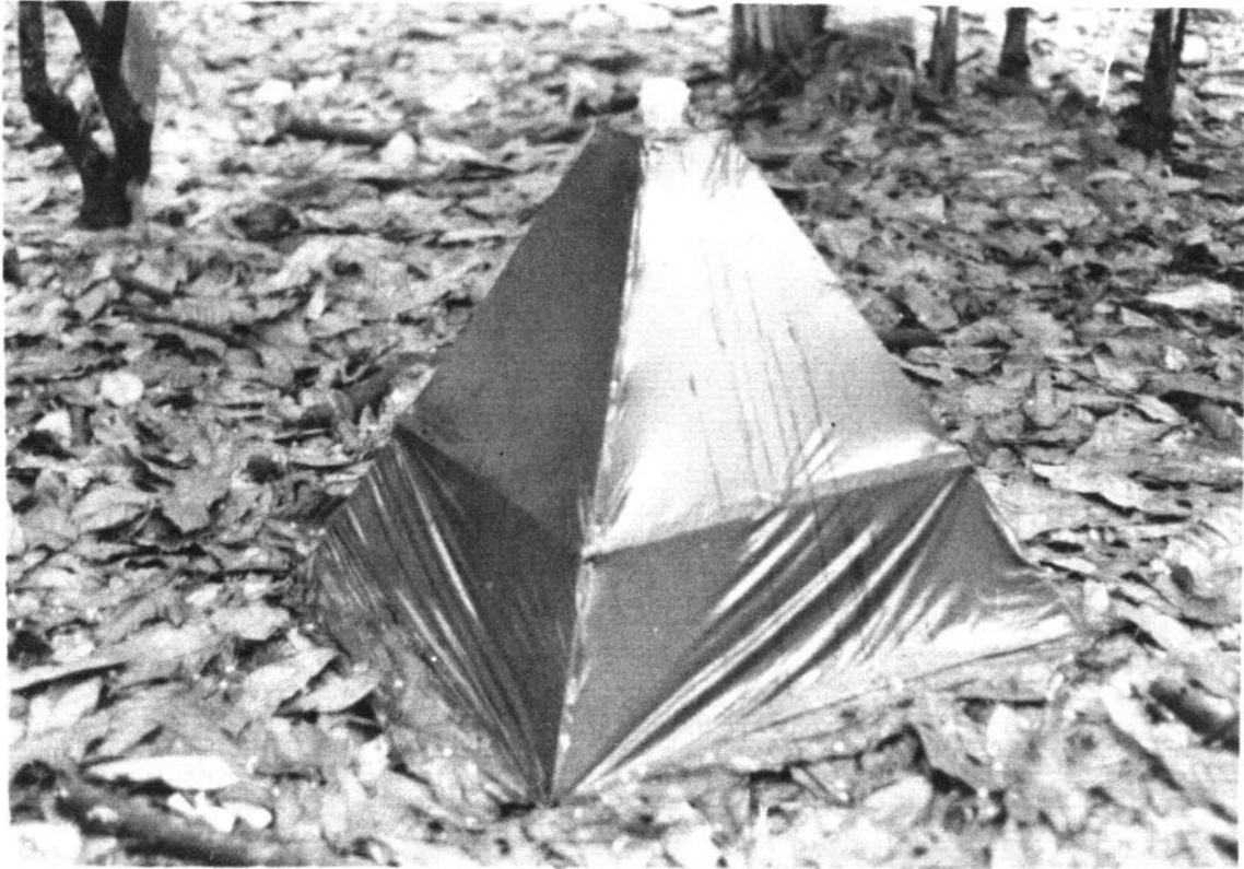
Photo 1 (above): A typical emergence trap (type A) used for sampling adult Culicoides as they emerged from decaying banana stalks. Three to five sections of banana stalks are covered by the trap. Photo 2 (below): Another type A emergence trap used to sample Culicoides midges emerging from discarded cacao hulls.
