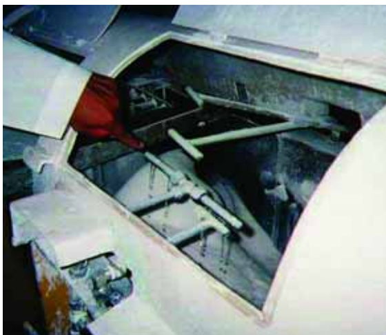
FIGURE 5.10 Wet method equipment: fluoride/iodide dosing mixture trickles down on salt in large capacity ribbon mixer.
