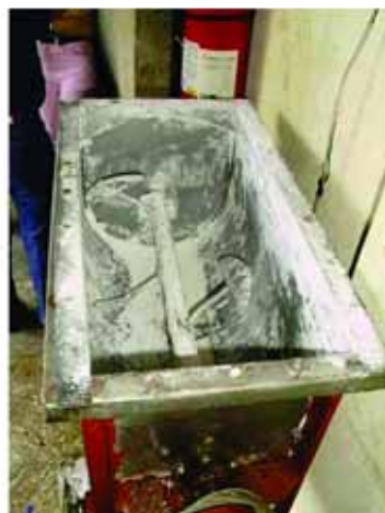
Figure 5.6 Dry method equipment: 500 lb capacity paddle mixer used for dry mixing of salt and fluoride and iodide additives.
