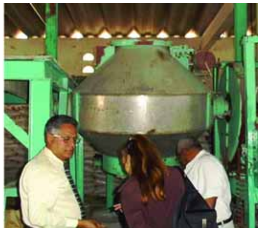
Figure 5.7 Dry method equipment: 2 ton capacity rotary mixer used for dry mixing of salt and fluoride and iodide additives.
