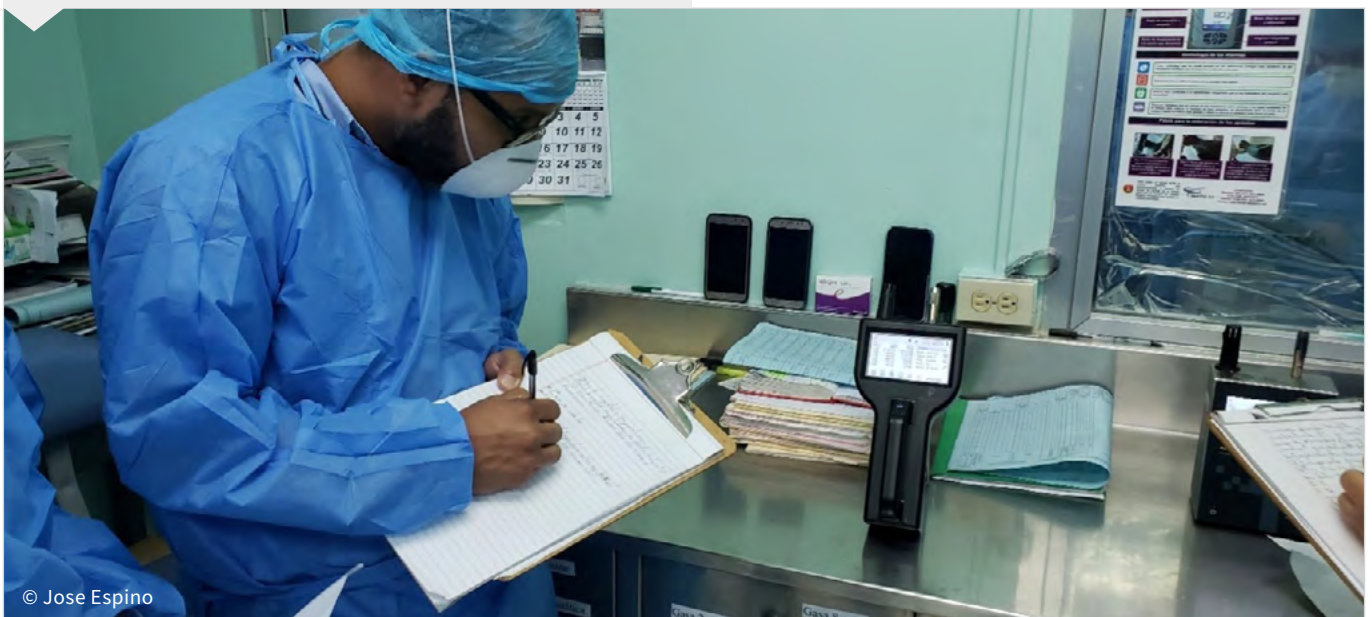
Figure 13. Assessment of cleanliness level with a particle counter in a clinical laboratory
