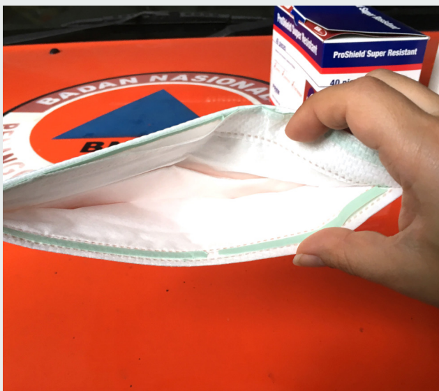
Figure 8. Perished N95-certified masks, previously donated to BPBD, Indonesia by an international NGO. The green 'line' towards the lower front of the mask was one of the head straps, but the elasticated material has disintegrated. Every mask had broken head straps.
