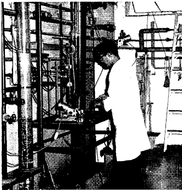
A pilot plant for research on filtering material for water treatment. The model, made of plastics, facilitates observation of the filtering process.
