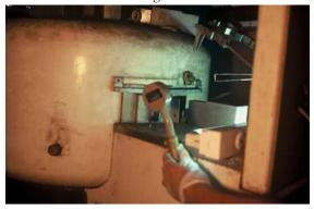
*Figure 40:* Checking activity of the radium sources before packing and removal.
