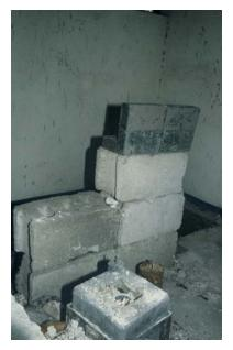
*Figure 27:* Improvised shield to test whether sources were leaking.
